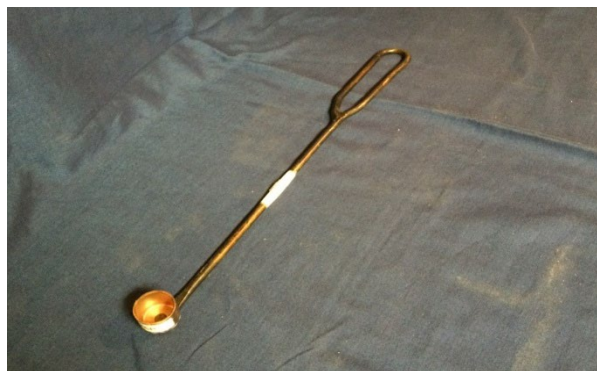
Figure 8. A long-handled bait dispenser can be constructed easily with a copper end cap, rivet, and ¼-inch rod. Compare the end-cap's capacity against a teaspoon cooking measurer to confirm correct volume.
