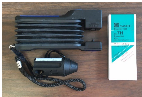
Figure 9. Hand-pump used to draw air into the glass testing tubes containing a chemical sensitive to the presence of phosphine gas.
