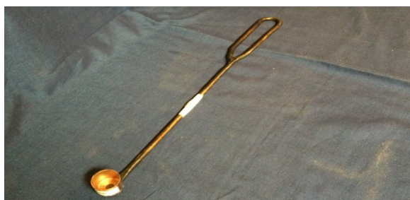
Figure 10. Bait dispensers can be made from copper pipe, split rivets, washers, and 1/4-inch rod. Match the capacity of the cut pipe with a baker's teaspoon. Label dipper "For pesticide use only".
