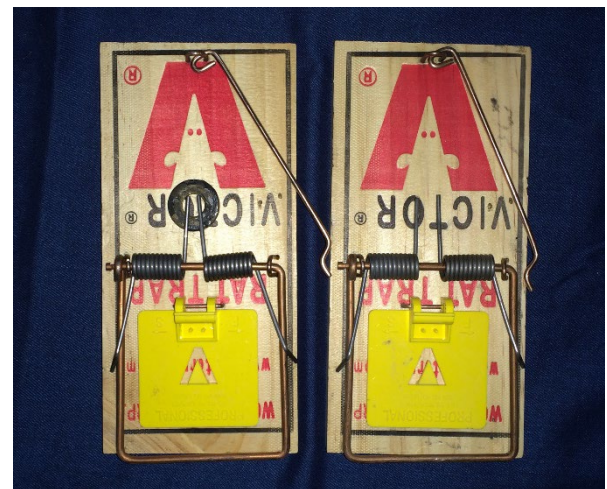
Figure 4. The left trap has a washer to under the spring tines to prevent them from embedding in the wooden base. This technique increases the trap's striking power (watch your fingers) and improves capture/kill rates.
