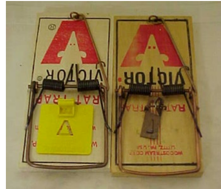
Figure 3. Expanded trigger (left) and traditional trigger (right) rat traps
