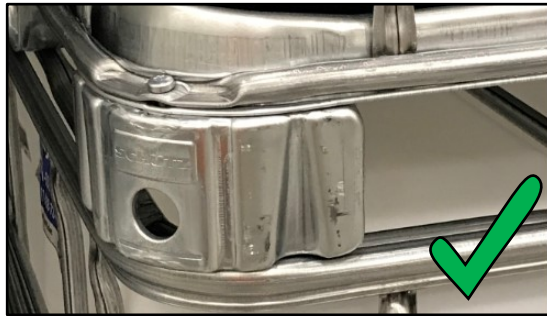
Corner foot is in good condition
