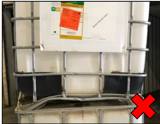
Frame is damaged
