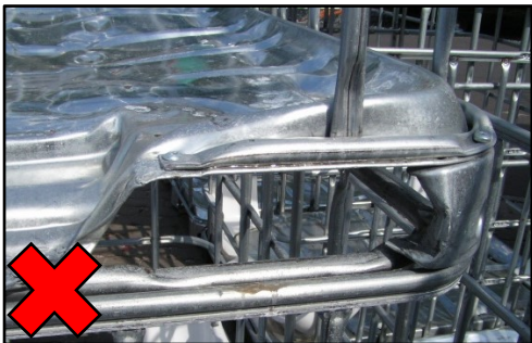
Corner foot is damaged
