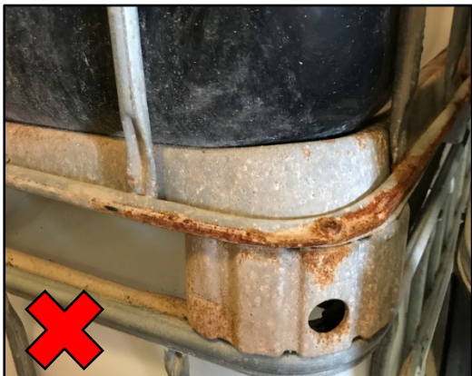
Corner foot is rusted
