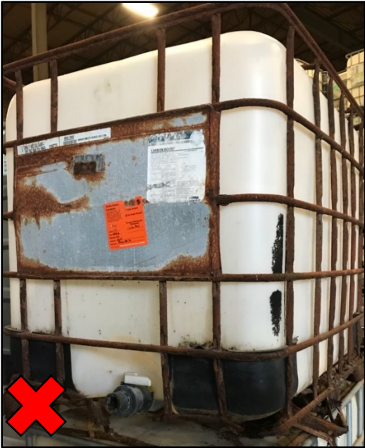
Entire frame of IBC is rusted
