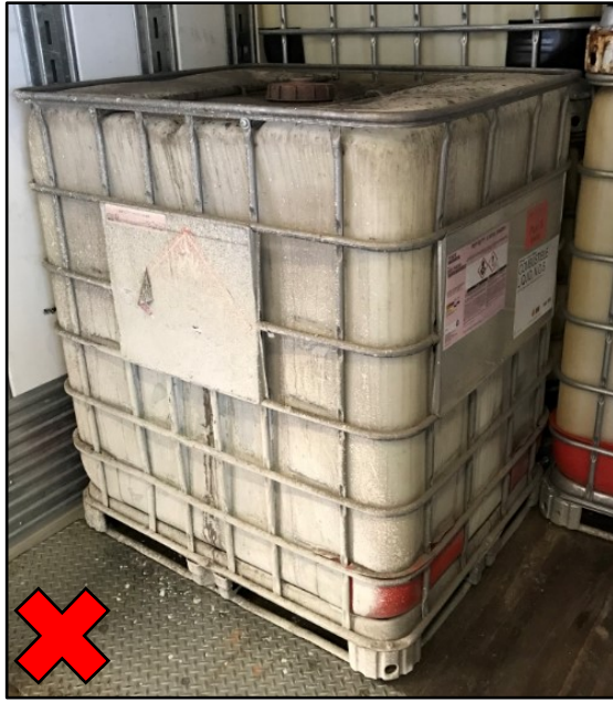
IBC has product residue on outside
