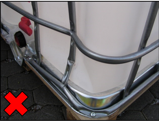
Frame is damaged
