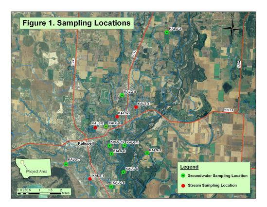
Samples collected during this project were taken to the MDA Analytical Laboratory Bureau at Montana State University and analyzed for 94 pesticide compounds (herbicides, insecticides, and fungicides) and nitrate. A summary of laboratory results are included in Table 1.
