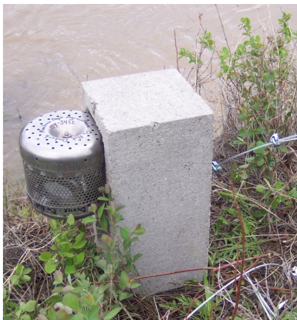
POCIS device ready for deployment
