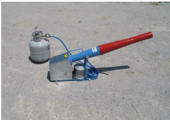
**Figure 7** Propane cannons can be scheduled to fire intermittently.
